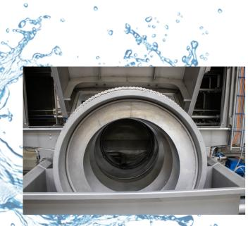
The High Pressure Label Remover (HPLR) removes different kinds of labels that are placed on the crate during its cycle in the supply chain. To make sure all kinds of labels are removed, Numafa used different configurations of pressure and nozzles within the HPLR.
